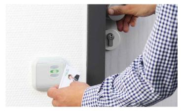
Within a system where the contact part is handled by people, it simply isn't possible to protect the electrical contact surface. Any contact based identification system will fail if there is something between the contact and the identifier.
